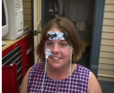
Figure 11. The typical hook up of Electro-oculogram (EOG) electrodes for BioPac Lab 10.
